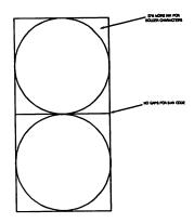
The combination of resolution, dot size and dot shape are elements in determining the print quality.
