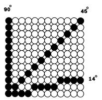
To achieve print quality using a raster device, the scalloped effect must be minimized. This can be accomplished using various techniques. The most straightforward technique is to control the distance between dot centers and thereby controlling the resolution (dpi). Raster hardcopy output devices vary in resolution from under 80 dpi to greater than 400 dpi.
