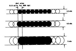
A third technique for minimizing this scallop effect is to alter the shape of the dots from round to square, as determined by the shape of the print stylus. Square dots minimize the scallop effect, providing more readable characters, and better line drawing and bar codes
