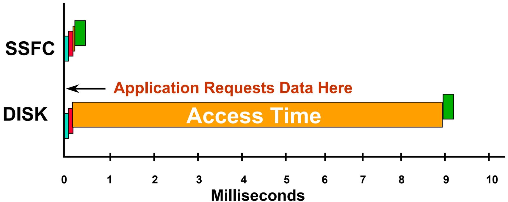
■ CPU overhead   ■ Controller overhead   ■ Access Time   ■ Data time
