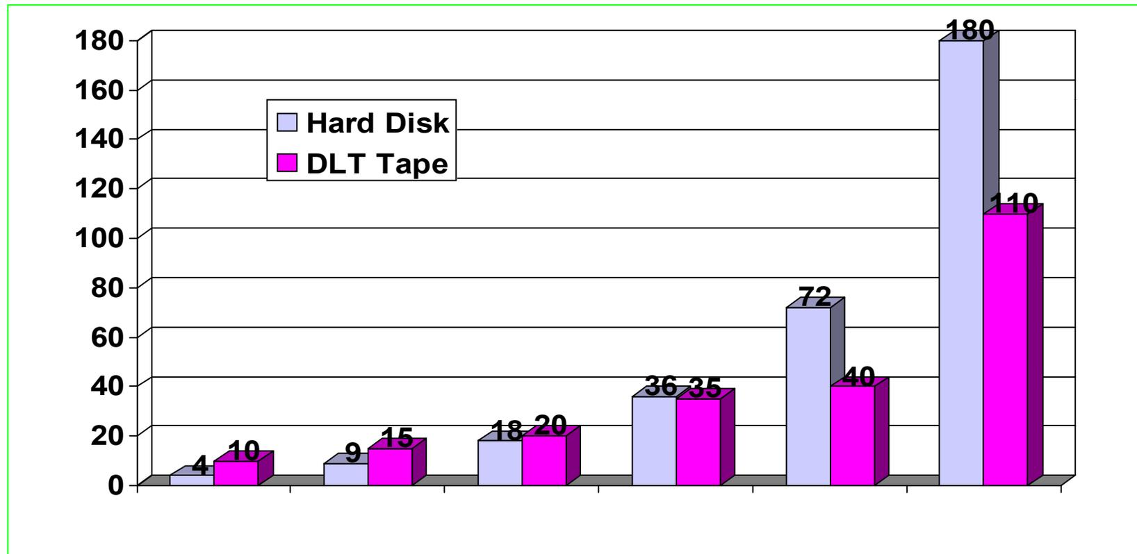
Tape drives used to be bigger than hard drives. This changed with the 36 gig drive.
