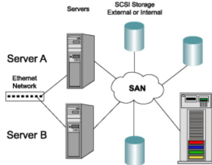
A SAN simply connects multiple hosts to a common set of storage devices.
