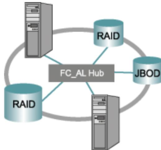
**Fibre Channel Arbitrated Loop (FC\_AL)**
